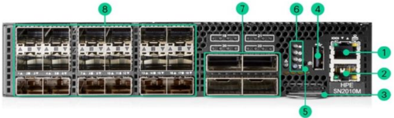
HPE Storage Switch M-series SN2010M (18 x SFP28 + 4 x QSFP28) Front View
